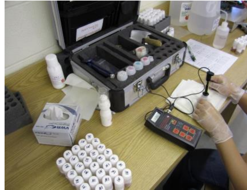
Drilled powder samples tested for chloride content (chemical testing)
