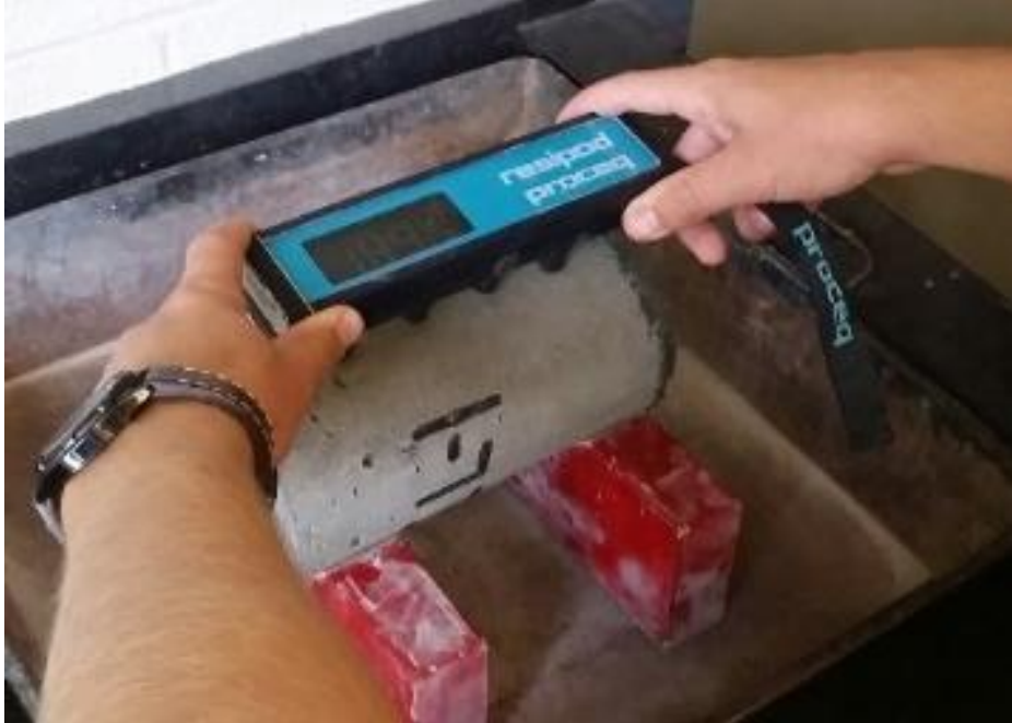
Resistivity testing for permeability (rapid electrical test)
