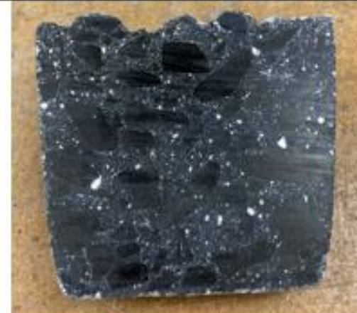
Figure 4.2b: Treated specimen prior to scanning. Note the presence of more air voids than in the specimen shown in Figure 4.2a
