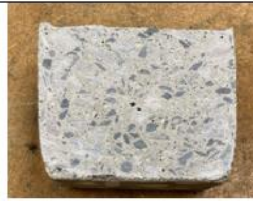
Figure 4.1b: Specimen sawcut, prior to polishing
