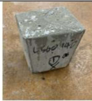
Figure 4.1a: Specimen cast for hardened air void analysis
