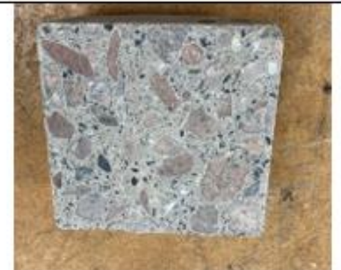
Figure 4.1c: Specimen after face is polished using progressively finer grit
