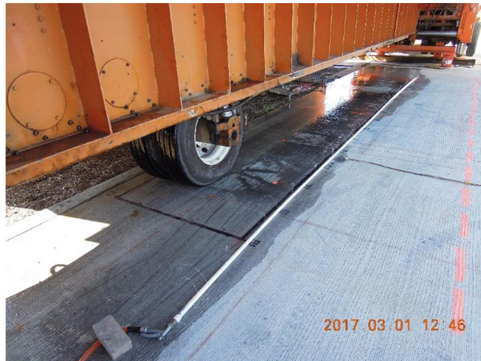
Continuous water supply during the flooded HVS testing
